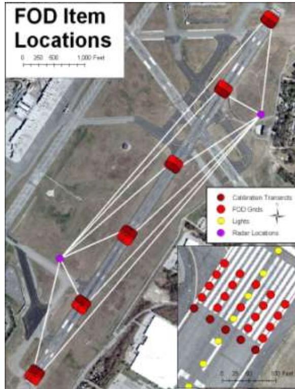
Figure 3. Location of FOD Arrays at PVD.
