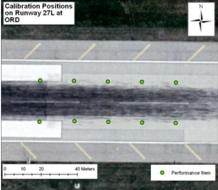
Figure 9. Performance Target Placements on Runway 27L At ORD.
