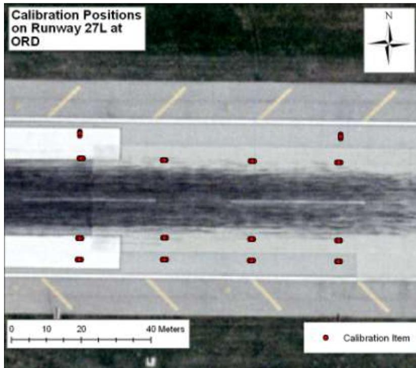
Figure 6. Calibration Target Placements on Runway 27L at ORD.
