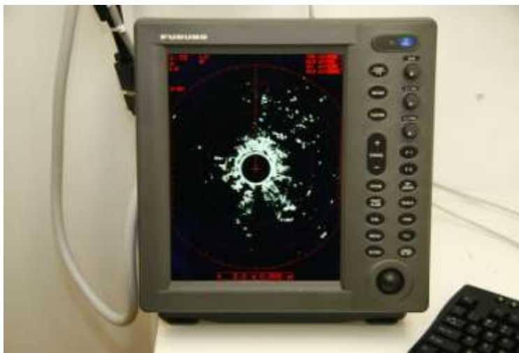
Figure 3. A Furuno ® Radar PPI.
